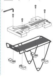
2 · Insert the four bolts into the holes in the top of the adapter (LT-40B) and screw them into the clamps (Clamp-B) on the underside of the adapter, as illustrated. Make sure the bolts are sufficiently tight to clamp the adapter securely to the rack.
